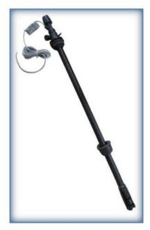
To complete the range of accessories for dosing stations, are available suction lances of adaptable length with connection for purge tube 4x6 (8x12 on request), complete with built-in non-return valve and level sensor, suitable for dosing stations with tanks up to 1000 litres.
